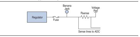
Table 2–31 summarizes the banana jacks and fuses associated with each power rail that can be supplied by external power.
