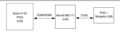
Table 2–25 lists the components used for the Ethernet port and the manufacturing information.
