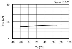
Current consumption vs. temperature in power-down mode
