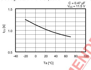
Overdischarge detection time vs. temperature
