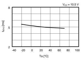
Overcurrent3 (load short) detection time vs. temperature
