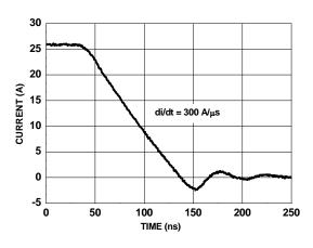
Figure 14. FDMS0306AS SyncFET Body Diode Reverse Recovery Characteristic
