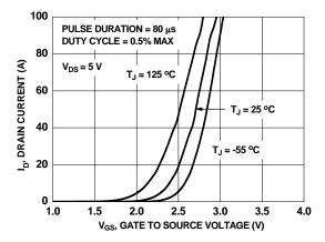
Figure 5. Transfer Characteristics
