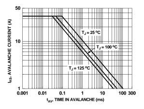
Figure 9. Unclamped Inductive Switching Capability
