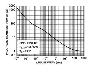
Figure 12. Single Pulse Maximum Power Dissipation
