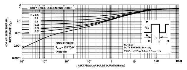
Figure 13. Junction-to-Ambient Transient Thermal Response Curve
