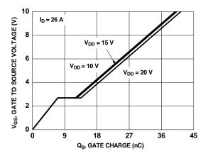
Figure 7. Gate Charge Characteristics
