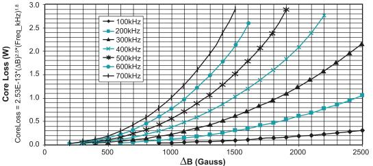
ΔB = 120E3 \* Vin\_min \* Dutycycle\_max / (Freq\_kHz \* Pri\_Turns)
