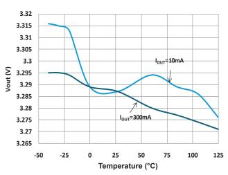
Fig. 13 Output Voltage vs. Temperature
