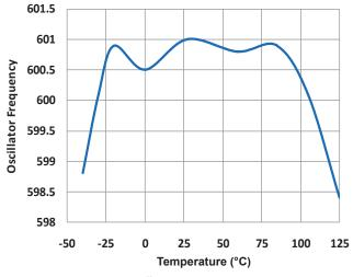
Fig.15 Oscillator Frequency vs. Temperature
