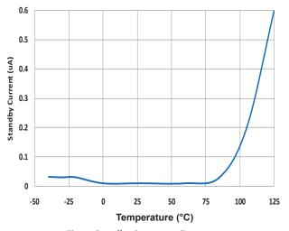
Fig.12 Standby Current vs. Temperature
