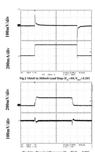
Fig.4 Line Transient Response ( $V_{\rm CC}$ =4V,  $V_{\rm OUT}$ =0.8V)
