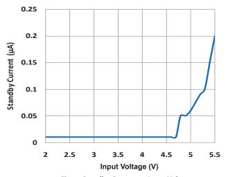
Fig.11 Standby Current vs. Input Voltage
