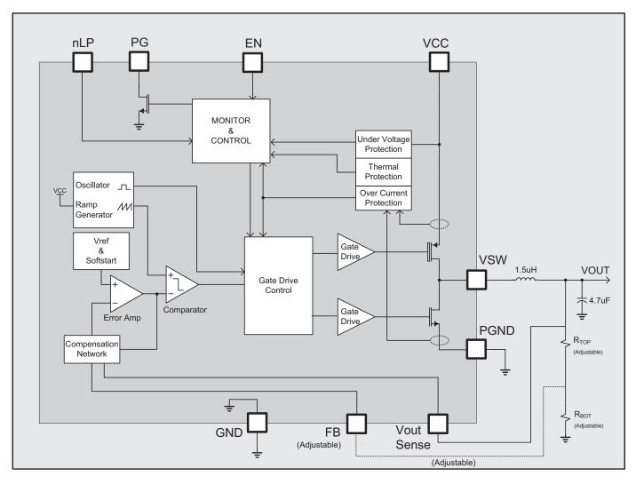
Figure 1: TS33000 Block Diagram for fixed and adjustable mode devices
