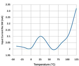
Fig.16 Input Current vs. Temperature (No load, No switching)
