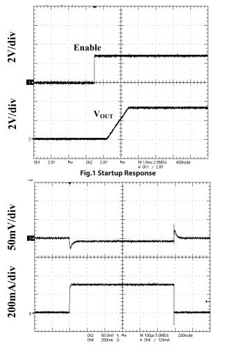
Fig.3 10mA to 300mA Load Step (V $_{\rm CC}$ =4V, V $_{\rm OUT}$ =0.8V)
