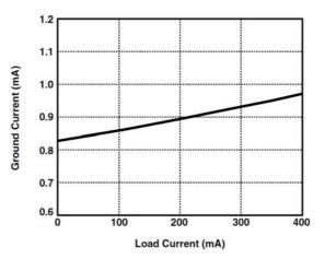
Figure 4. Ground Current vs. Output Load
