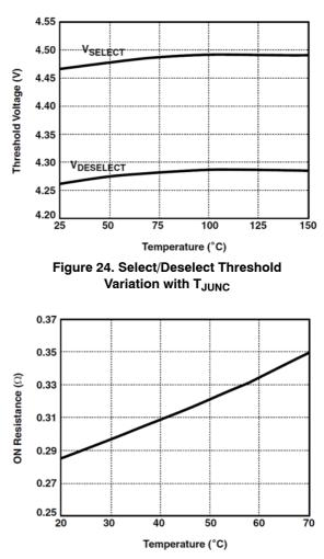
Figure 25. V<sub>AUX</sub> Switch Resistance vs. T<sub>AMB</sub>
