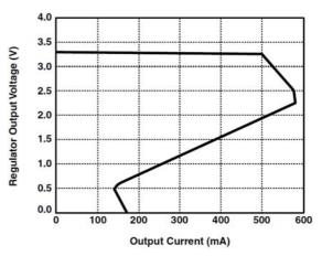
Figure 8. Foldback Current Limit Protection
