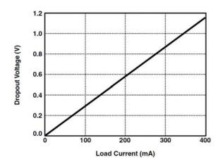
Figure 9. Regulation Dropout Characteristics
