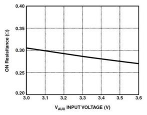
Figure 10. Switch Resistance vs. V<sub>AUX</sub> Supply
