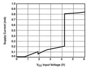
Figure 1. V<sub>CC</sub> Supply Current vs. Voltage
