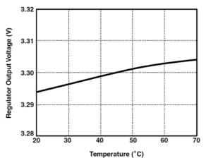
Figure 23. V<sub>OUT</sub> Variation with T<sub>AMB</sub>(400 mA Load)<sub>T</sub>
