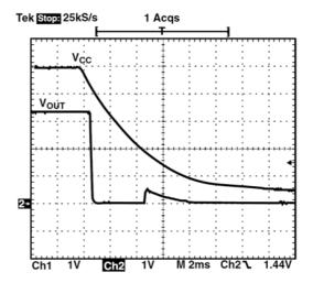
Figure 12. V<sub>CC</sub> Full Power Down (Load = 400 mA)
