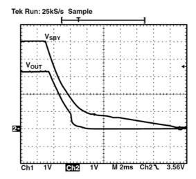
Figure 14. V<sub>SBY</sub> Full Power Down (Load = 400 mA)
