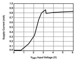
Figure 2. V<sub>SBY</sub> Supply Current vs. Voltage
