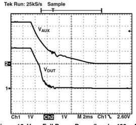
Figure 16. V<sub>AUX</sub> Full Power Down (Load = 400 mA)
