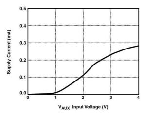
Figure 3. V<sub>AUX</sub> Supply Current vs. Voltage
