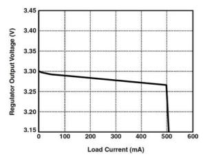
Figure 7. Load Regulation (5 V Supply)
