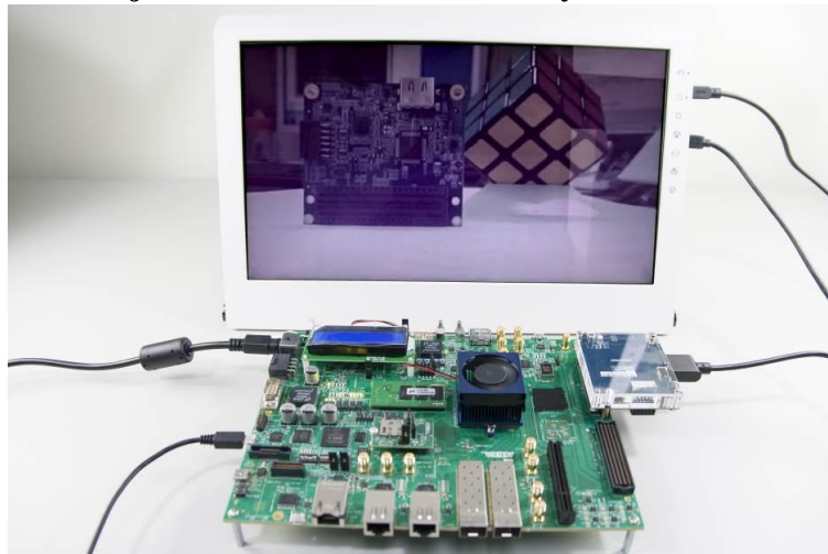
Figure 5-10 A10SoC_D8M_FMC_VIP demonstration running on A10SoC
