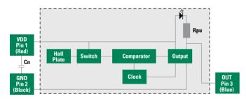
1. Add capacitor Cn as shown, close for the sensors for transient suppression if required.
