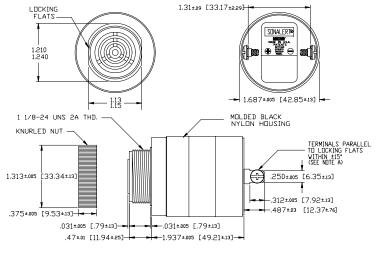
NOTE A: TERMINALS-.032 BRASS TIN PLATED, TAPPED FOR #6-32 SCREW. TWO #6-32 NICKEL PLATED BRASS SCREWS INCLUDED. WILL ACCEPT 1/4' QUICK CONNECT. NOTE B: MOUNTING- REMOVE BLACK PLASTIC NUT AND INSERT THREADED FRONT THROUGH 125' HOLE PUNCHED IN PANEL, IF DEKENTATION IS NEEDED, NOTE LOCKING FLATS ON DRAWING. SCREW NUT BACK ON. DO NOT DVERTIGHTEN.
