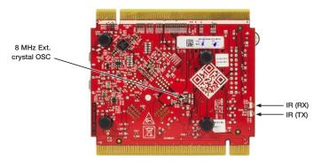
Figure 2: Back side of TWR-KL43Z48M module
