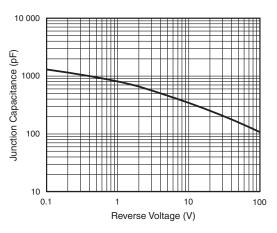
Fig. 5 - Typical Junction Capacitance Per Diode
