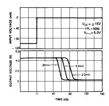
Figure 8. Response Time for Various Input Overdriver
