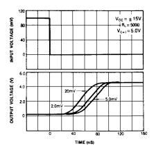
Figure 7. Response Time for Various Input Overdriver
