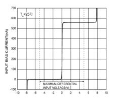
**Figure 6. Input Characteristics**
