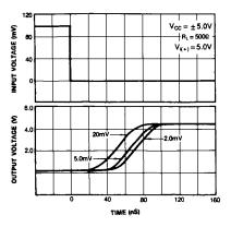
Figure 5. Response Time Various Input Overdriver
