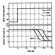
Figure 4. Response Time for Various Input Overdriver
