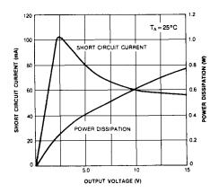
Figure 12. Output Limiting Characteristics
