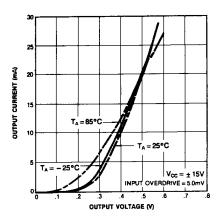
Figure 2. Output Saturation Voltage
