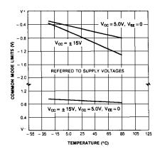
Figure 11. Common Mode Limits
