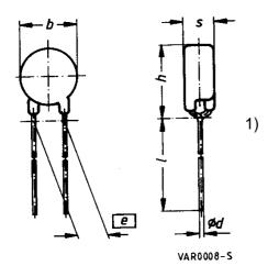
$b_{max} = 12.0$   $b_{max} = 17.5$   $s_{max} = 7.5$   $e = 7.5 \pm 0.8^{2}$   $0.8 \pm 0.05$
