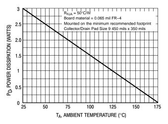
Figure 15. D<sup>2</sup>PAK Power Derating Curve
