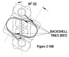
**CAUTION:** Make sure the cable assembly is pushed all the way forward into the front shell so that it is retained by the Backshell after crimping.
