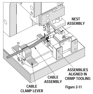
Warning: Once the press ram handle has started to descend, it cannot be returned to the up position until the full stroke of the press has been completed. In case of a jam or some other problem, should the press ram ever need to be returned to the up position, before completing the full stroke, pull up on the ratchet release lever and raise the press ram handle. The ratchet release lever is located on the upper left side of the press frame. See Figure 2-3.
