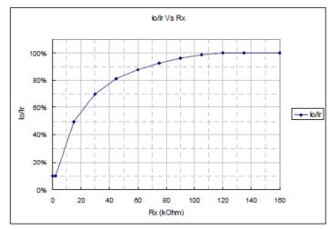
**Dimming Configuration using External Resistance**
