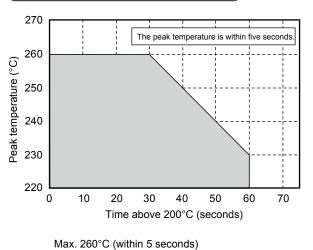
The times of repeated reflow soldering must be two times or less. The Temperature must be measured at top of the cell.
