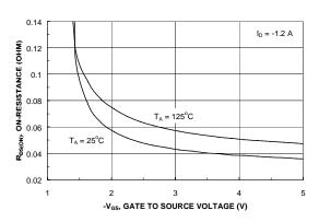
Figure 3. On-Resistance Variation with Temperature.
