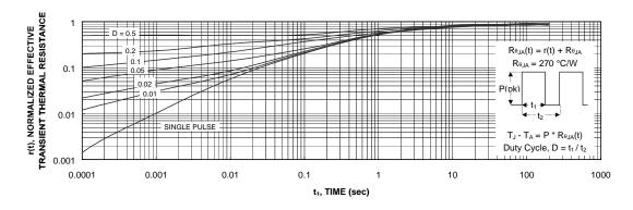
Figure 11. Transient Thermal Response Curve.
