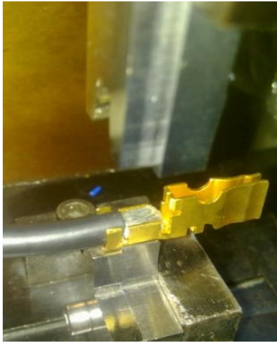
Picture 5. Position before Crimping Picture 6. Positon after crimped
