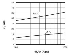
Fig. 7 - Typical Stored Charge vs. dl<sub>F</sub>/dt
